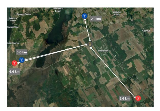
Along with "Shadowing" from surrounding buildings and/or topography, a network's signal degrades over space. The further away from the tower, the weaker it becomes.
