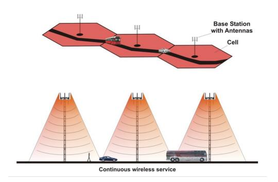
This illustration demonstrates how towers work to create a continuous wireless service that is constant and reliable.
